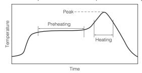
For lead-free soldering (Example: Sn/Ag/Cu)
